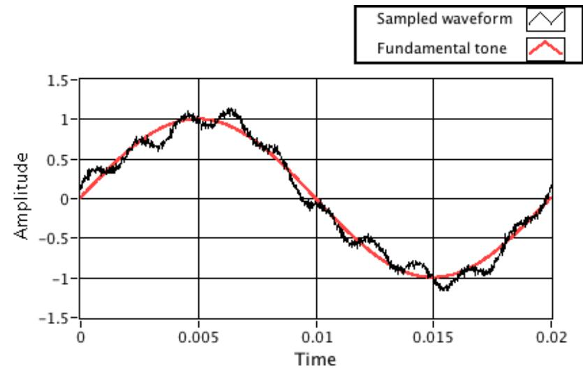
**Observation:** in the real world the sampled waveforms are always distorted and with time-varying frequency.
