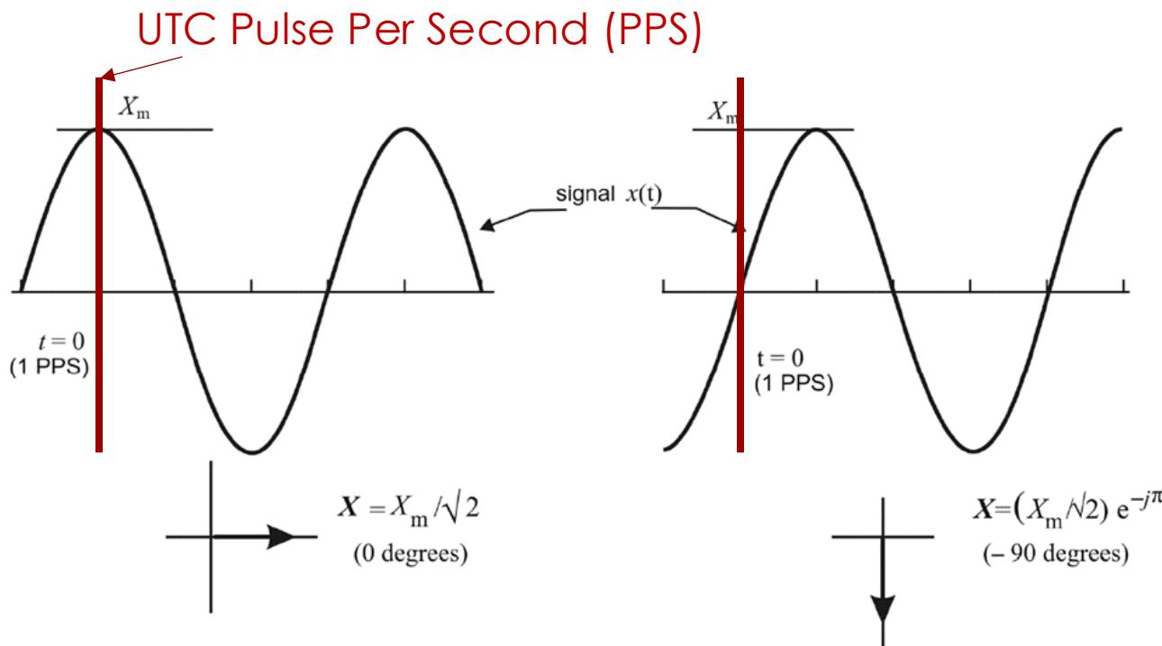
**IMPORTANT:** the common time reference is fixing the reference phase.
