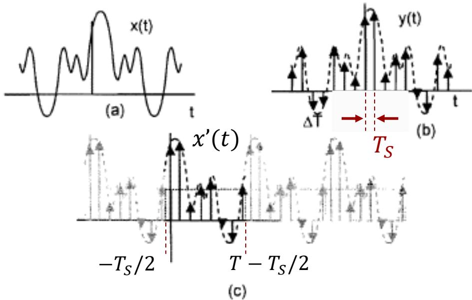
Note that, **although the original function  $x(t)$  was, in general, not periodic, the function  $x'(t)$  is periodic and we may consider this function to be an approximation of  $x(t)$ .**
