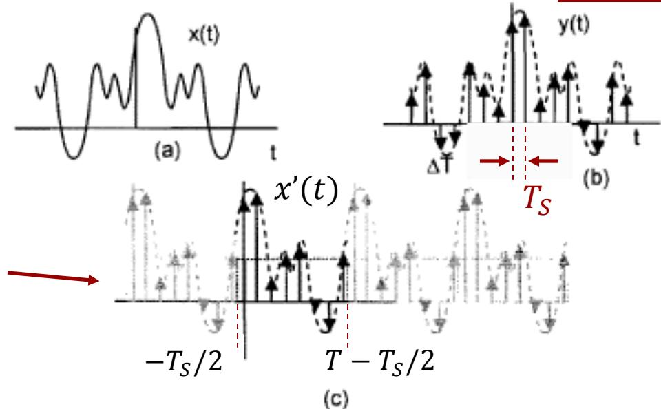
Since the limits on the integration span is of one period only, we may remove the summation on  $m$ , and set  $m = 0$ , thus using only the samples over the period shown in bold in figure (c). Therefore, the previous equation becomes
