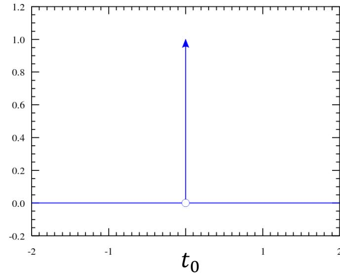
The impulse function is a **sampling function** in the sense that when the integration of the following equation is performed, the result is the sampled value of the function  $x(t)$  at  $t = t_0$ :
